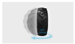
**Differential Steering**Provides better energy efficiency and agile maneuvers, including the ability to rotate on the spot and make tight turns.
